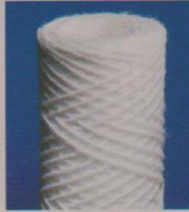
Multilayer 405 Cartridge braided cop with layers of different loops, food-grade polypropylene, quality of filtered water: 20 microns.
